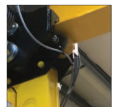
Reaction Roller counter balance for chain containers over 10mtr height of lift.
